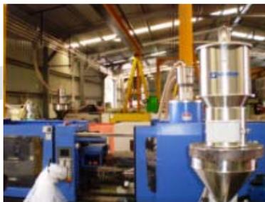
Sunshine Plastics are plastic injection moulders operating since 1978 on the Sunshine Coast, Queensland. In 2008 Sunshine Plastics installed a Labotek central materials handling system incorporating a desiccant dryer to service their higher output machines.
