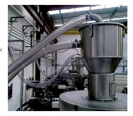
stainless steel AISI 304, equipped with a remote vacuum valve with spring return, 50.8 mm T-pipe, level switch, coarse wire screen in lid, non return flap, and vacuum and material connections in 50.8 mm. Bottom cone is 60° with Ø80mm outlet.
