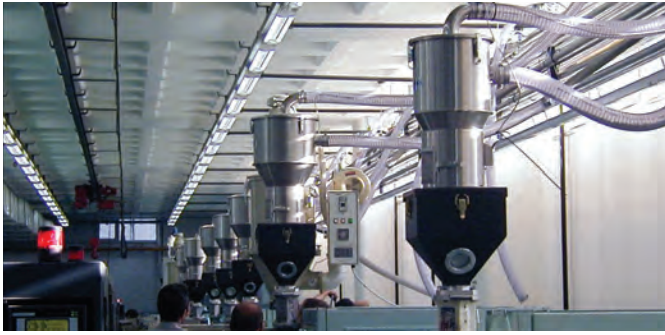
Vacuum receivers type SVR and insulated hoppers
