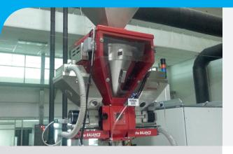
The MCWeight is specially designed to measure the actual feed capacity of an extruder. It has an integrated weighing module to accurately measure throughput and an integrated knife valve to control the filling.
