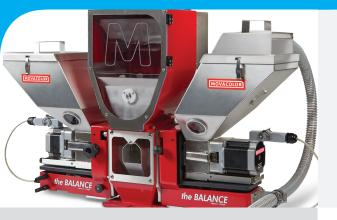
The MCHybrid\* is a unique dosing concept that combines two technologies into one system: batch blending and in-line dosing.
