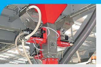
Advanced blending systems are often seen as complete plant engineered solutions. Movacolor has developed a unique modular system that allows you to put together a full gravimetric continuous blending system. Up to 15 components can be controlled from one controller. These systems can be installed on one extruder or on multiple co-extruders, creating a control platform for multiple continuous blenders in one system.
