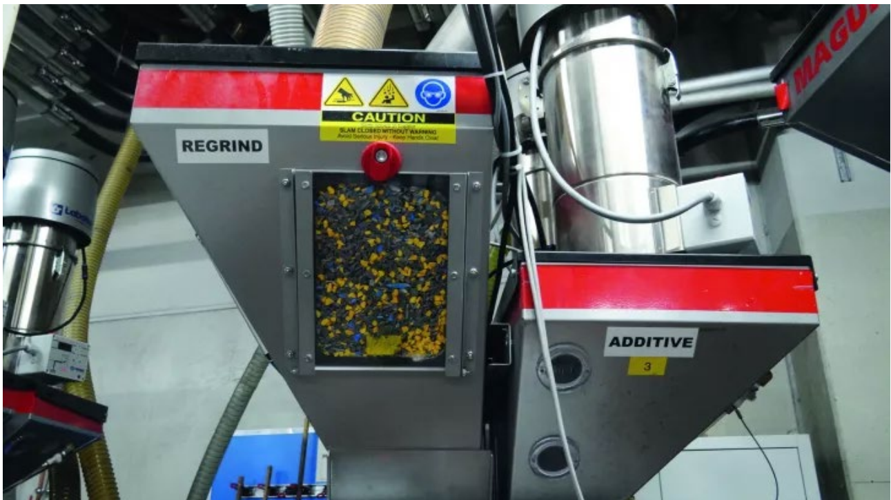
The gravimetric mixers enable precise dosing of the raw materials. (Image: editorial team).
