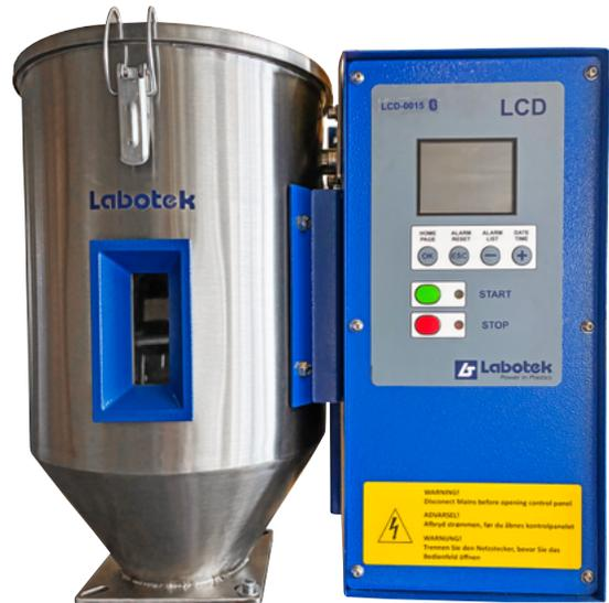
*The electronic control panel allows easy programming via the internal data base of main materials.*
