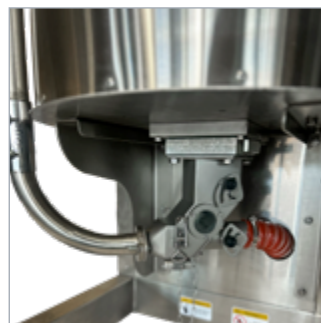
Injector with clean-out door
